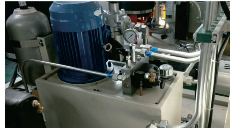
100L优质碳钢油箱，隔离双油箱设计 10L预充氮蓄能器溢流阀，安全阀，手动泄压阀压力变送器 100L tank, separate design and fillet inside. 4L accumulator, 100Bar Nitrogen Pre-Charged Pressure relieve valve, manual release
