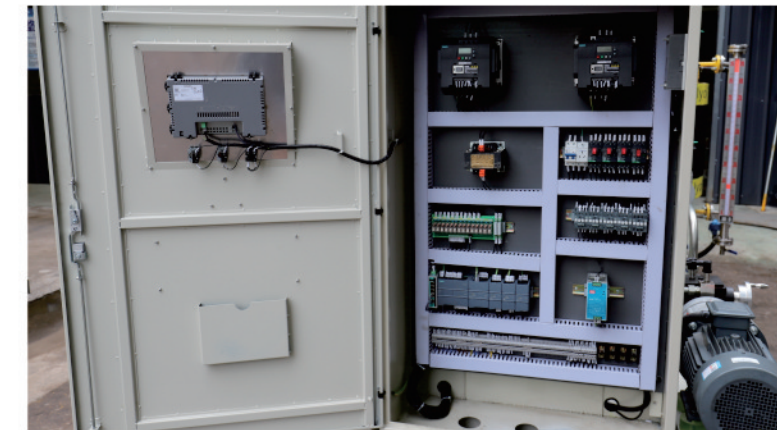
所有高压发泡机都采用变频器控制，省电在30%以上 All high pressure foaming machine adopts frequency converter control, save electricity above 30%
