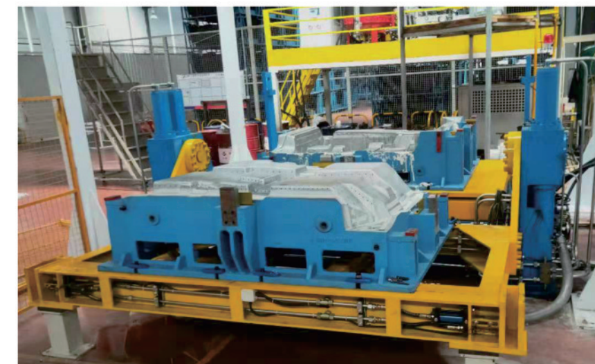
液压翻转模架 Hydraulic flip formwork
