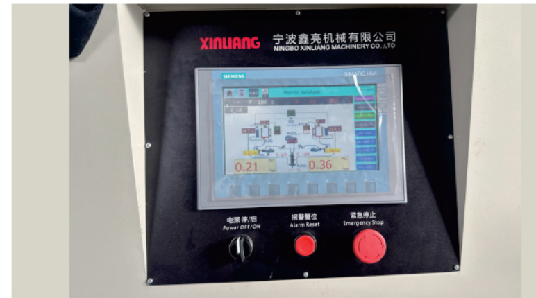
所有高压发泡机都采用10寸大触摸屏，原料温度压力料位显示直观， All high pressure foaming machine use the 10 inch touch screen, Raw material temperature and pressure level display intuitive
