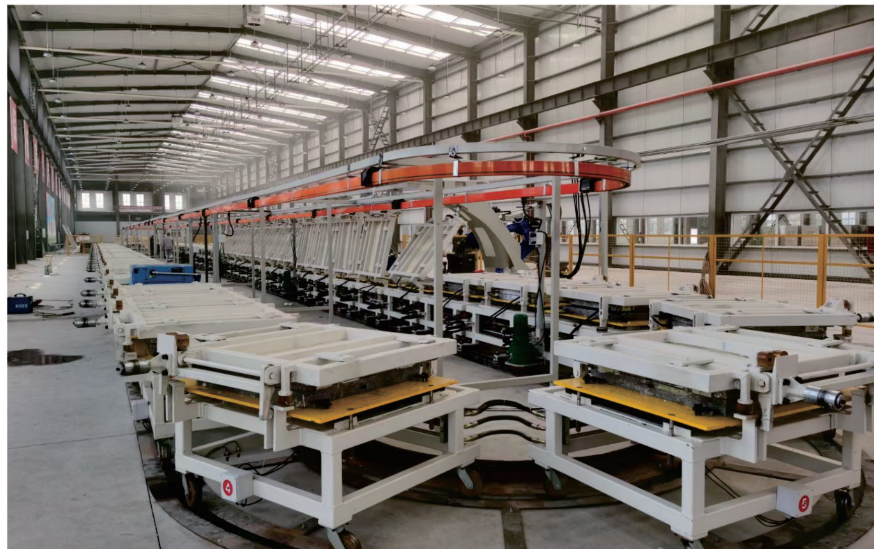
70工位全自动开合模发泡环形线 70 station automatic opening and closing mold foam ring line
